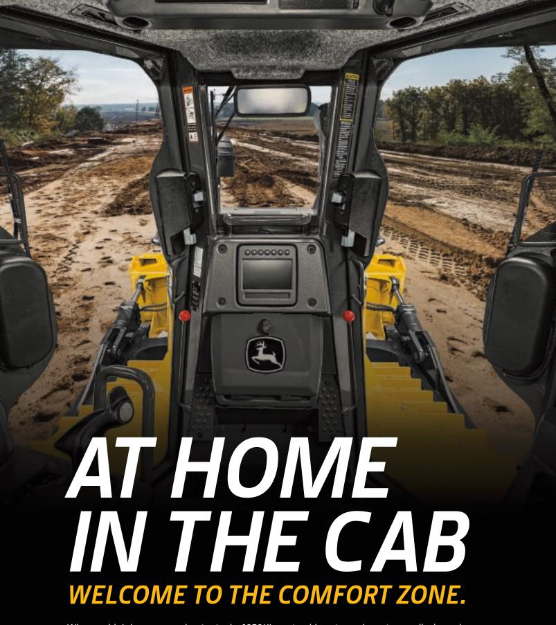
Who wouldn't be more productive in the 1050K's noticeably quiet and spacious walk-through cab? This dozer is loaded with all the fatigue-beating amenities an operator needs to get "in the zone" and get more done, including a new suspended double-bogie undercarriage that reduces vibrations in the cab by up to 75 percent, smoothing the ride over rough terrain.
