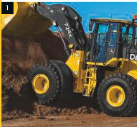
1. New adaptive clutch cutoff automatically provides more power to the hydraulic system, ensures smooth control at high engine rpms and low speeds, and allows for better machine handling in all terrain without the operator having to change settings.
