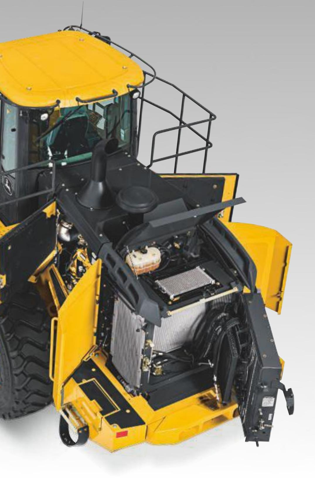
Greasing is less messy thanks to centralized lube banks that provide easy access to zerks. Conveniently located periodic lube and maintenance chart confirms that nothing gets overlooked.
