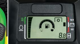
**Easy-To-Read Display** Includes an electronic fuel gauge that provides real-time fuel level information. There's even a tachometer with best cut target zone.
