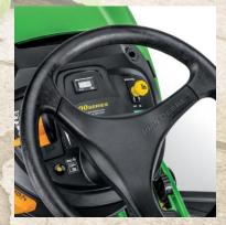
**Electric PTO**, available on some models, provides instant engagement of mower blades. Ignition switch and single lever throttle/choke are on the dash within easy reach.
