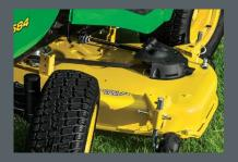
Accel Deep" Mower Decks Designed to mow fast well, the deeper "draw" and flat top design create a better quality of cut at faster ground speeds.
