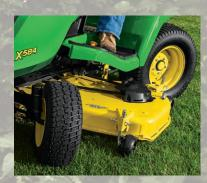
Four-Wheel Steer. All four wheels turn in unison around obstacles for extra tight turns. (Available on the X354, X384, X394 and X584 Select Series.)
