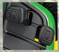
Twin Touch System. Twin Touch" automatic transmission lets you easily change from forward to reverse with two-pedal foot control for effortless speed and direction changes. (Available on the X300 and X500 Series.)
